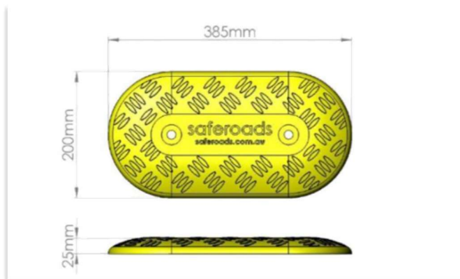
Figure 4 - Pavement Bar Example
