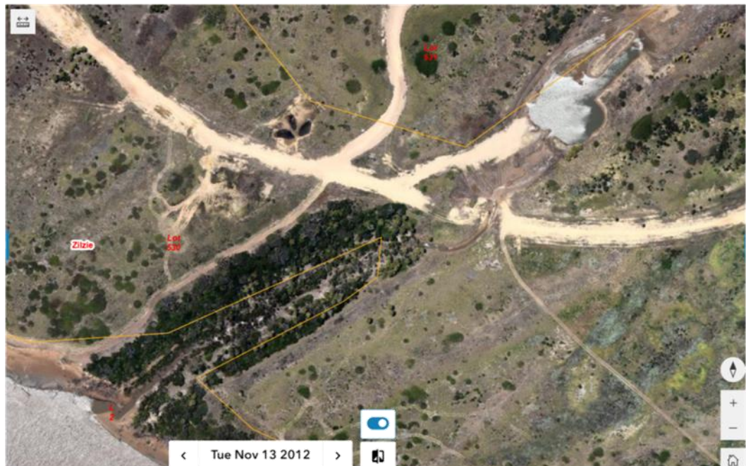
2012 - still no connection, but large borrow pits excavated along the drainage path
